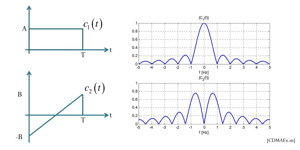
The two waveforms above overlaps both in time domain and in frequency domian.
